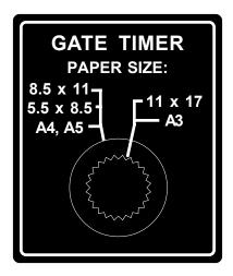
For 11" x 17" paper, set the knob as shown. The knob can be left in this position for any other paper size with feed rates up to 2,300 booklets per hour. For faster feed rates with smaller paper, turn the knob to the 8.5x11 position.
