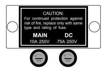
Lift open the front guard. The fuse panel is located on the left side wall. Use a small screw driver to open each fuse holder.
